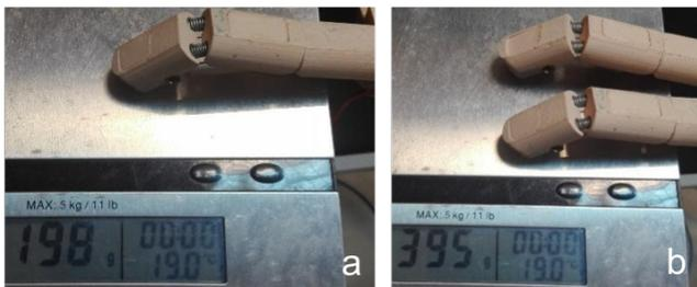
Fig. 10: Normal forces exerted by the fingertips of the prosthetic hand.
