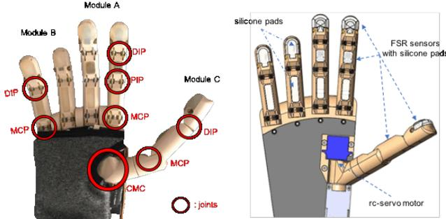
Fig. 2. CAD model of the developed prosthetic hand
