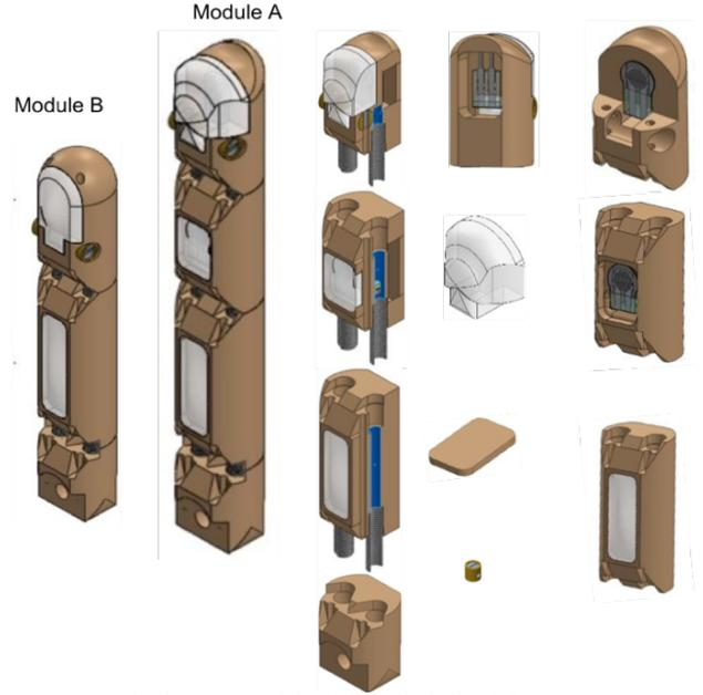
Fig. 3. CAD models of the robotic hand fingers.
