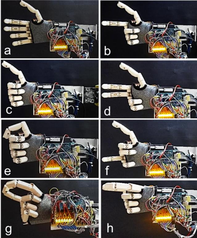
Fig. 8. Several gesture patterns made by the prosthetic hand.
