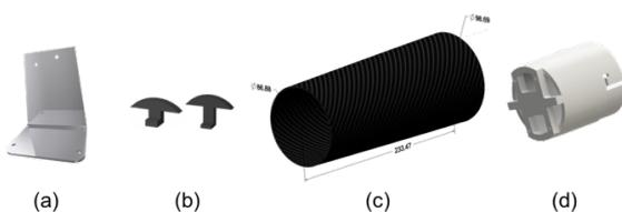
Fig. 6. The CAD models of the parts comprising the forearm: (a) the internal support plate, (b) the two wedges, (c) the external carbon fiber case and (d) the internal base as connected to the prosthetic hand.
