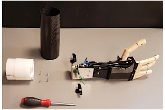
Fig. 7. The manufactured parts of the forearm and the prosthetic hand.
