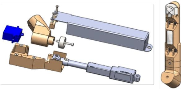
Fig. 4. The CAD model of the underactuated thumb with its actuators.
